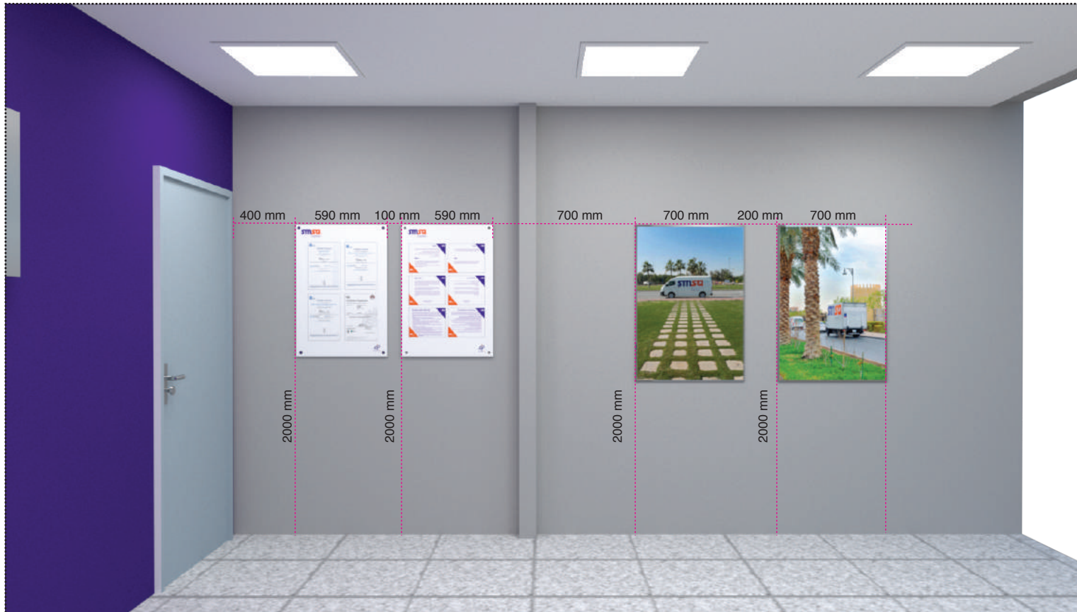
Reverse printed acrylic and wall graphic instalation guide
