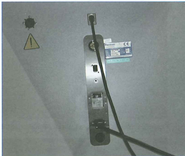
Figure 9: 620XR End Panel, Circuit Breaker, IEC Socket
