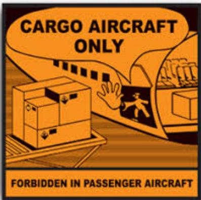
Packages or overpacks of Dangerous Goods bearing the “Cargo Aircraft Only” label must be loaded in accordance with one of the following provisions;
