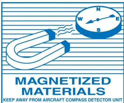
MAGNETIZED MATERIALS are Cover materials with relatively high magnetic field strength such as magnetrons and non-shielded permanent magnets without keeper bars installed. Masses of ferro-magnetic metals such as automobiles, automobile parts, metal fencing, piping and metal construction material, even if not meeting the definition of magnetized materials, may be subject to operator's special stowage regulations since they may affect aircraft instruments, particularly the compasses.
