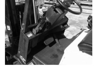
Shake the overhead safety cage to ensure it is firmly bolted to the forklift. Note any
