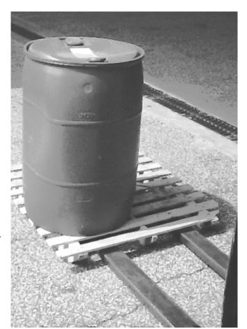
Here, the operator has engaged the same load by driving under the skid to one side. Not the preferred method; however, more of the drum's center of balance is over the blades. The operator has a better chance of getting this freight to its destination.
