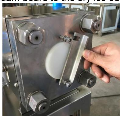
and then press and hold "LCO<sub>2</sub> feed" for about 8~12 seconds, to let the raw material into the dry ice machine generator cavity. At this time, gas will be discharged from the "exhaust port", and dry ice will be generated. The dry ice snowflake is left and cool the cavity. This is called "pre-cooling".
